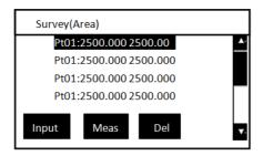
2.Press soft key 'Input' to transfer coordinates from coordinate file or enter the coordinates manually with keyboard, otherwise press soft key 'Meas' to measure the coordinates of the target point. The coordinates are all listed in the screen and the maximum number of points when Area Surveying is 20. The inputted and measured coordinate is inserted below the indicator column, which determine the shape of the formed area.
