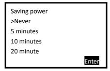
You may choose 'Never' to set off auto shutdown. When choosing 5, 10, 20 minutes opts, the instrument will automatically shut down after chosen time if there is no key pressed. Use  $\blacktriangle \lor$  keys to move indicator '>' up and down to the wanted opt. Press soft key 'Enter' or ENT to save the setting. Pressing ESC will result in no changes of settings.
