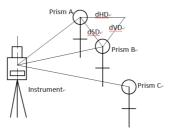
Measure the horizontal distance (dHD), slope distance (dSD), elevation difference (dVD) and azimuth angle (dHD) between two target. You may also enter the coordinate or transfer coordinate from files to calculate the value above out.
