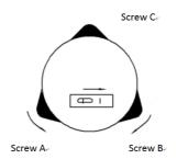
③Turn around the instrument by 90  $\degree$  again. Repeat the process in  $\frac{1}{2}$  and  $\frac{2}{2}$  until the bubble remains centered (leveled) at all sites.
