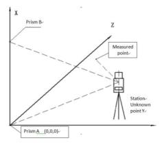
The function serves to measure the length (X), distance (Y) and altitude difference (Z) the prism deviates from the baseline origin and the baseline.
