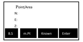
Press 'F2' to list out all coordinates in the current measurement file. Press 'F3' to list out all coordinates in the current coordinate file. The function explained above works in all pages inputing NEZ coordinates.
