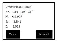
Now turn around the aiming component of the instrument to aim at the offset point. Mention that the offset point must be on the defined plane but not below the prism bar for concerns of precision.
