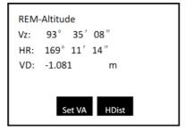
4. Then turning the telescope up and down. The elevation difference between the target and the reference point is displayed in the VD column.
