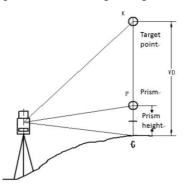
There are two modes for REM measurement: 'with TH' and 'without TH'. Users may select 'with TH' mode when altitude from ground to target is to be measured, otherwise 'without TH' when altitude from any reference point to target is to be measured.
