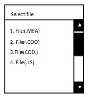
Each file involves operations of 'establish new files' (New), 'delete files' (Del) and 'view'(View) which is called File management here.
