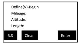
Enter the mileage, altitude and length one by one and press 'ESC' to end the input and go to 'List of V curve'. The uses of 'Save', 'View' and 'Edit' $\rightarrow$
