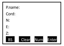
Using keys '♣' helps to scan the sequence of each point. e.g'1' indicates the number of the point when it is recorded or scanned. After setting up one record, press 'ENT' to accept the setting and enter the setting page of the next record. If do not need record any more, press 'ESC' to quit 'Input coordinates' function. The system will now ask users if he or she wants to save the record. After choosing 'save', the record will be saved into coordinate files.
