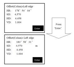
Aim at the left edgeand press soft key 'Enter' Enter 'Offset(column)—Right edge'. Aim at the right edge and press soft key 'Enter'
