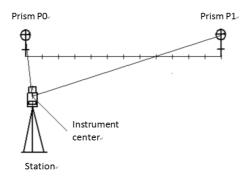
When undertaking equidistant stake-put, users may first measure the coordinate of the origin/begin (prism P0) then that of the terminal/end (prism P1).
