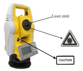
Warnings: See directly into laser beams constantly is destructive.
