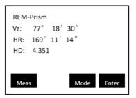
3.Aim at the prism and press soft key 'Meas' to obtain the horizontal distance of the target from the instrument. Press soft key 'Enter' to enter 'REM-Ground to target'
