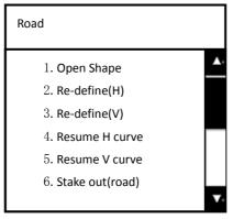
If you have already imported LS files into the instrument from the external, then you may open the [.LS] file through '1.Open Shape file'. Users may choose from three opts after opening the LS file: 'Stake-out roadway', 'Resume H curve' or 'Resume V curve'.
