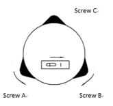
2 Turn the instrument around about the vertical axis by90 and re-center the bubble
