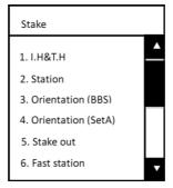
The '<u>Setup Station</u>' and '<u>Orientation (BBS)</u>' are the preparation work for staking out. If users have already setup station and orientation of BBS, re-setting them are not necessary.
