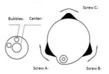
4)Using tubular level to level the instrument precisely
