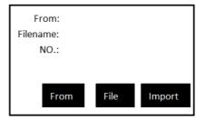
If the current coordinate file is saved in the flash memory the instrument, the name of it is the "filename" by default. Press the "From", and then press the "Select" to select ".txt "file under the corresponding directory, which is desired to be imported in the file list of U disk. For example, if we select the file of 0712.txt,press the "File" button to choose file of coordinates which you want to import (there you can create a new file) such as SVY.COO, then the interface is shown below:
