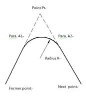
The system will not accept negative Para. A1, Para. A2 nor Radius R. If inputting the radius, then the system will insert arc with defined radius in between the former point and the next point. If inputting parameters A1 and A2 of the spiral, then the system will insert defined spiral in between the line and the arc. [Notes\*]: When inputting A1 and A2 according to the length of the spiral L1 and L2, the formulae to calculate A1 and A2 are as followed:
