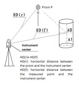
When measuring the coordinate of the earth point A1 of the projection of AO, set up the instrument height and target height.
