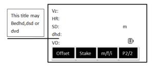
>dhd is to stake out horizontal distance difference. A positive result indicates that the measured horizontal distance is greater than the evaluated one. The lens should be shifted to the instrument.
