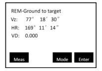
4. Then, turn the telescope up and down to aim at the target point. The VD column displays the elevation difference from the ground to the target point.
