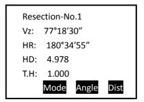
Choose angle or distance to undertake resection. If choosing angle mode then the instrument will start measuring distance. After a successful measurement, the system will display 'Next P'
