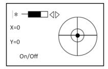
Adjust reflector by pressing 'left' key(►). Each time a left key is pressed, reflectance target is switched between prism (Prism), no-prism (NP) and reflector board (RB).
