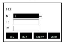
Setting up BBS is to relate the coordinate of earth station to the coordinate of the instrument (being used together with <u>STA</u> <u>Function</u>).
