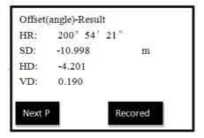
Now turn around the aiming component to aim at the offset point.
