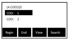
Select the points with the help of keys  $\blacktriangle \lor$  and press 'ENT' to save the your choice. If cannot get the point, the coordinate will remain its origin and the instrument will display 'Can't be get!'.
