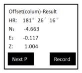
Now press soft key 'Next P' to enter the offset measurement of the next point; press soft key 'Record' to save the coordinate of the offset point.
